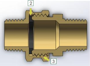
1 pipe thread 2 'O' -ring 3 outside diameter of 1.0625 and 11-1/2"threads per inch
